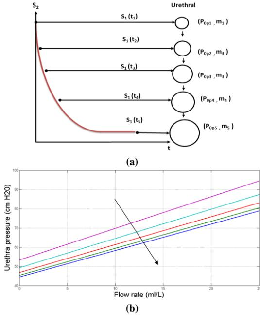
**Fig.4:** a) Urethral relaxation in response to nerve signals. b) Urethral Resistance Relation (URR) change in response to nerve signals. The arrows shows the direction of increasing relaxation .
