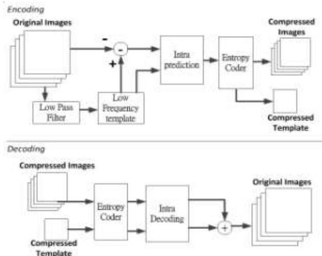
Fig.3.Low frequency template based compression block diagram
