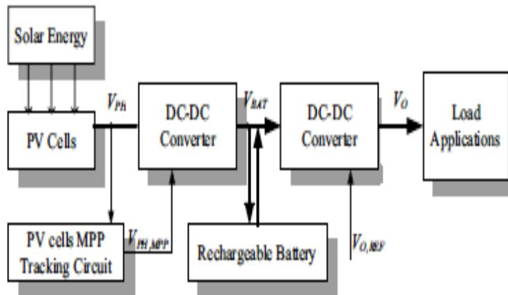
Fig. 1. Conventional Solar Power Management System
