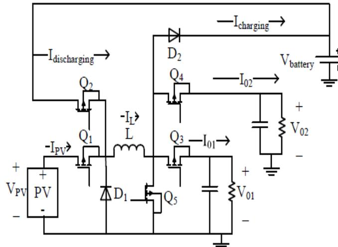
Fig. 3. The single inductor DIMO DC-DC converter
