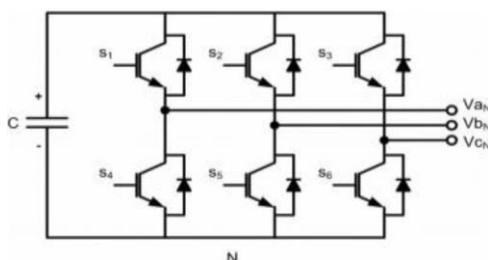
Fig. 4. Topology of Three Phase Inverter
