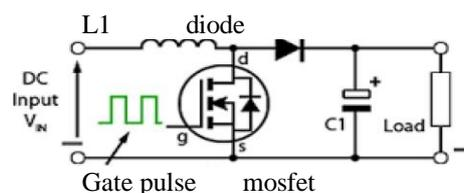
Fig.3. Boost Converter Circuit
