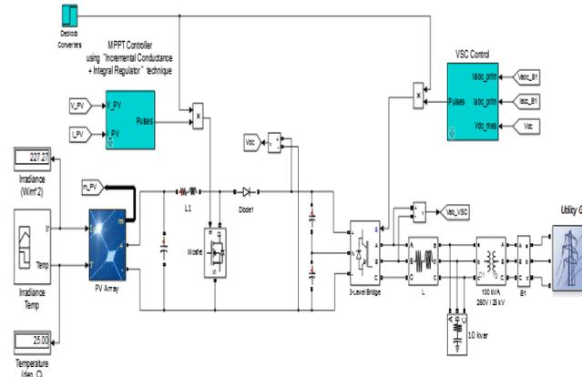
Fig. 5. MA TLAB model of grid-connected PV system
