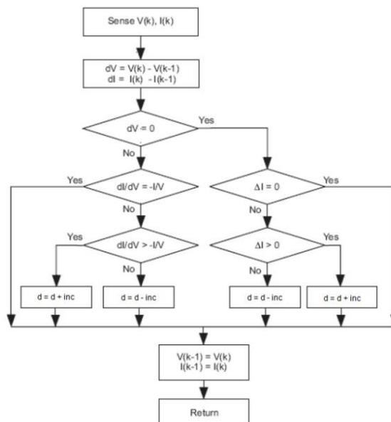
Fig.7. Flow chart incremental conductance algorithm
