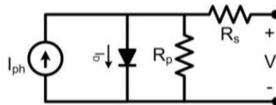
Fig. 2. Equivalent circuit of photovoltaic cell
