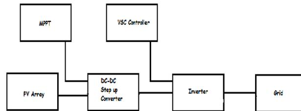
Fig.1. Grid connected PV system block Diagram
