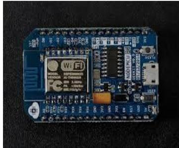
Fig 2- NODEMCU
