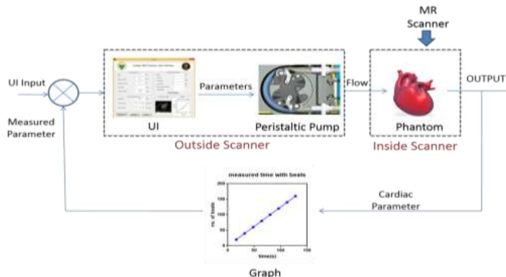
**Figure1:** Block diagram of the Cost Effective 3D Printed Cardiac Phantom
