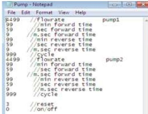
Figure 7: Different input parameters for Peristaltic Pump
