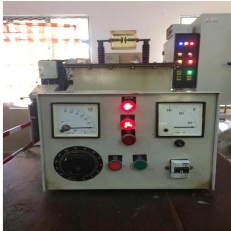
Fig1: Breakdown test apparatus
