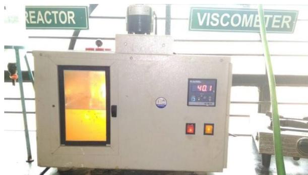
Fig2: Cannon –Fenske viscometer
