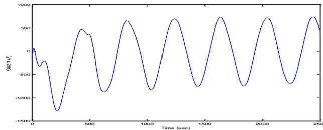
**Fig 4.2(a). Waveform of source side current with STATCOM**
