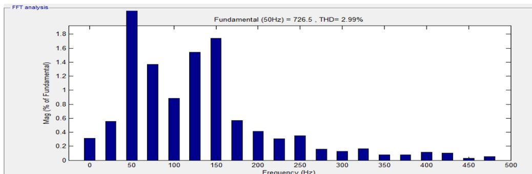
**Fig 4.2(c) THD of source side current with STATCOM**
