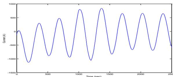
**Fig 4.1(b) waveform of load side current without STATCOM**
