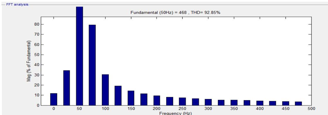
**Fig 4.1(c) THD of source side current without STATCOM**
