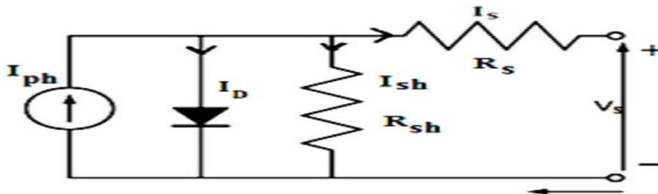
Fig 1. Equivalent Circuit of a Solar Cell
