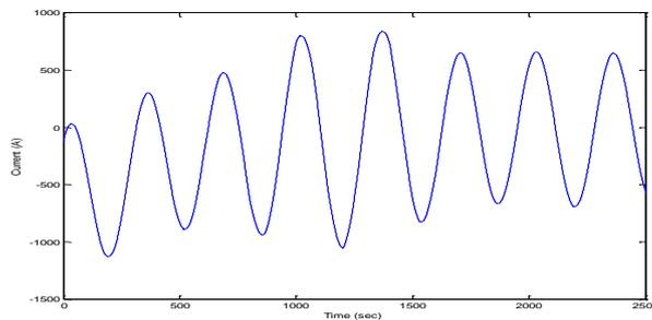
**Fig 4.1(a) waveform of source side current without STATCOM**
