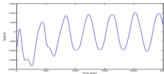
**Fig 4.2(b) waveform of load side current without STATCOM**
