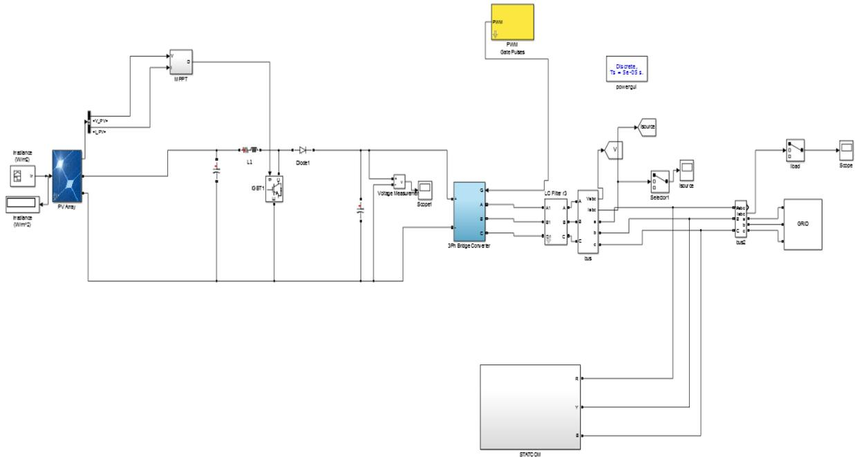
**Fig 4.2 Simulink model with STATCOM**
