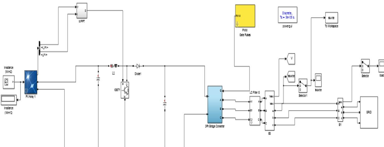
Fig 4.1. Simulink model without STATCOM
