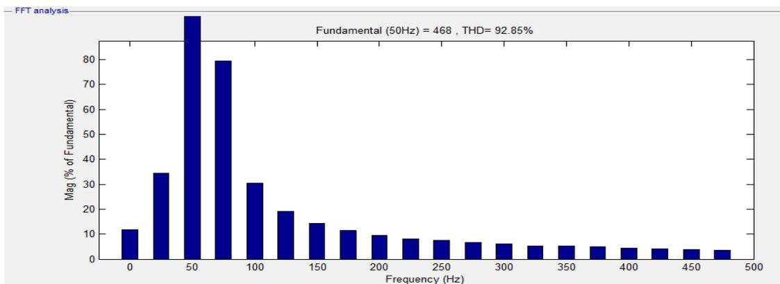
**Fig 4.1(d) THD of load side without STATCOM**
