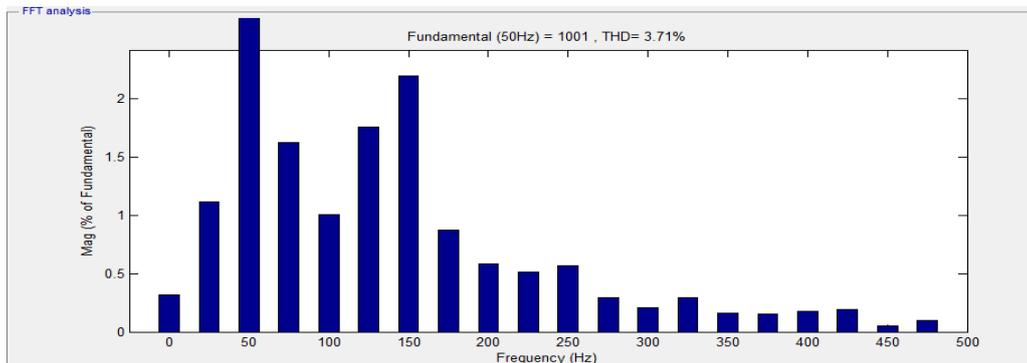
Fig 4.2(d) THD of load side current with STATCOM
