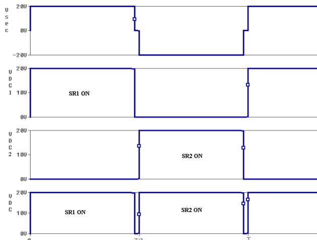
Fig. 4 Ideal timing for SDRS circuit
