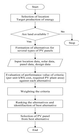
Fig.1: Flow chart for selection of PV panel.
