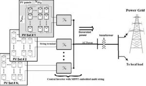
Fig.4 Battery less grid tie PV electricity generation system.
