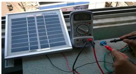
*Fig: Multimeter connected to PV panel*
