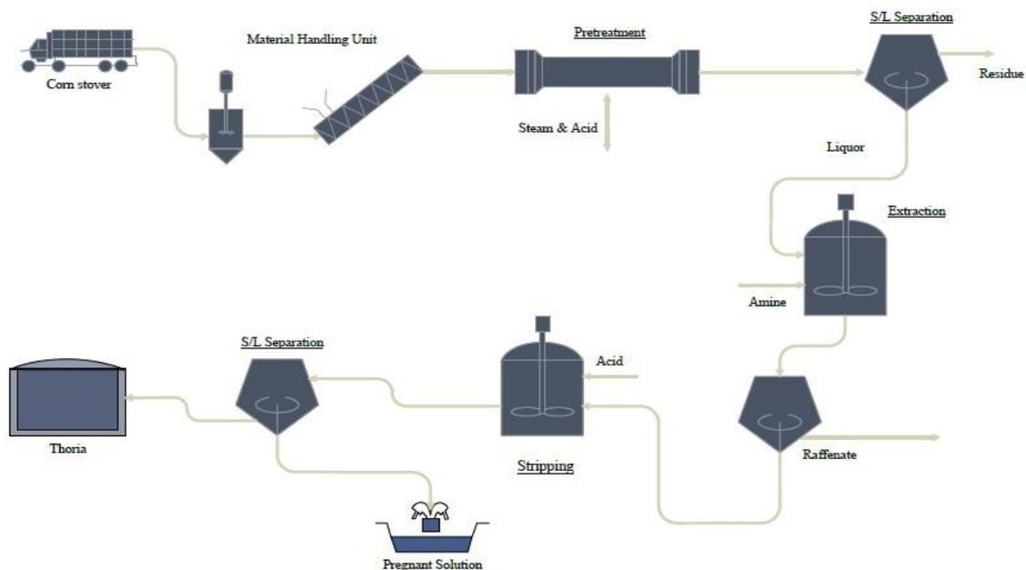
Fig 2 Process Flow Diagram of Thorium Extraction
