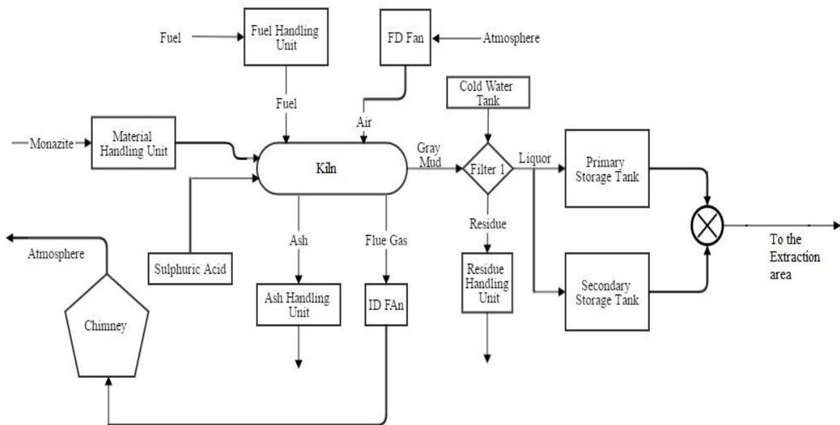
Fig 3 Plant layout of Pretreatment and Material handling unit
