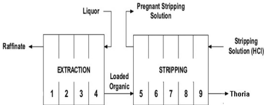
Fig 1 Flow diagram illustrating the successive extraction and stripping stages
