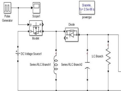
Fig.6 Buckboost Converter
