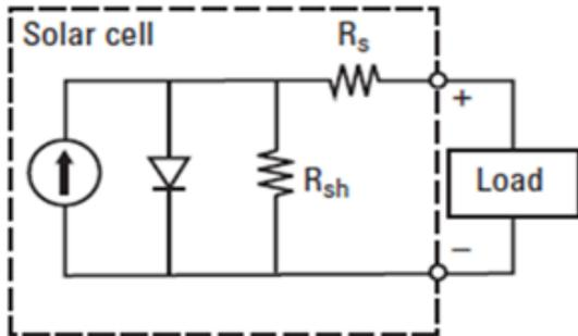
Fig 2: Single Diode model of the PV cell
