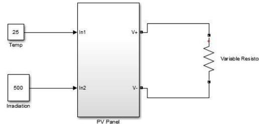
Fig. 3 Simulink model of the PV Panel
