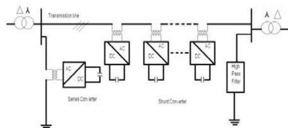
**Figure-7.** DPFC-distributed power flow controller.
