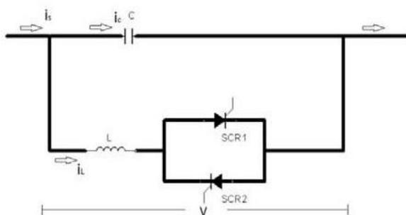
Figure-3. TCSC- Thyristor controlled series capacitor.
