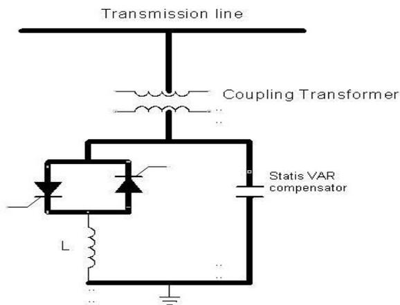
Figure-2. SVC- Static VAR compensator.
