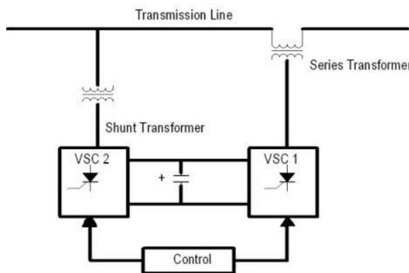
**Figure-5.** UPFC-unified power flow controller.
