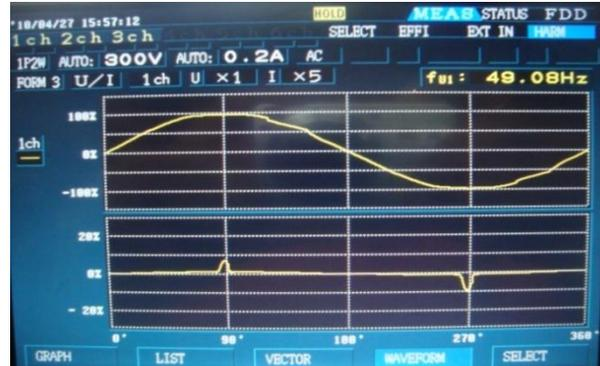
Figure 5: waveform for Mobile Charger
