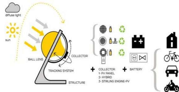
Fig.3 Working of Spherical Sun Power Generator
