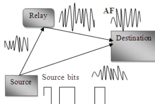
Fig.5 Amplified and forward
