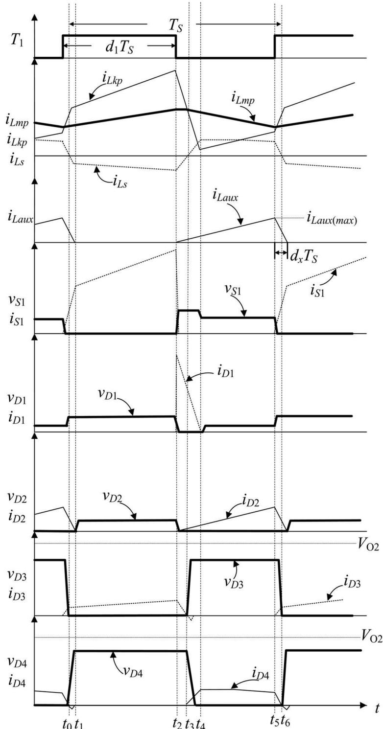
Fig. 3 Characteristic waveforms of high-efficiency SIMO converter
