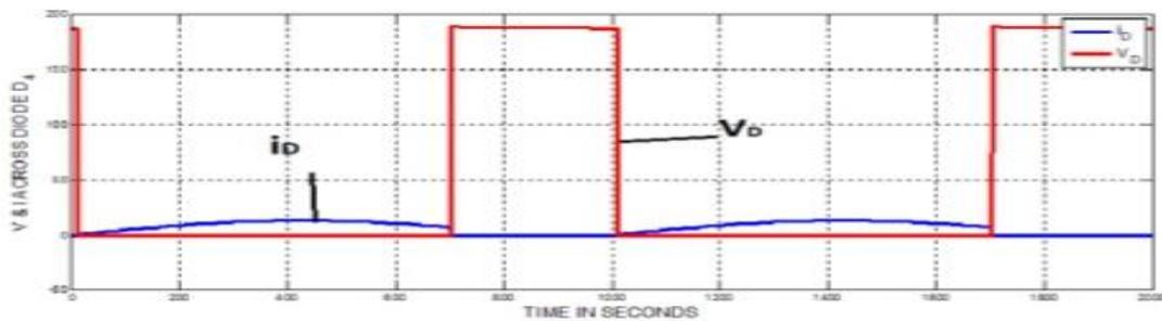
7.3 Voltage & current waveforms across switch
