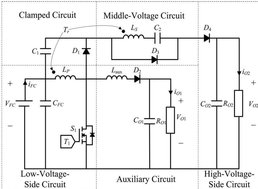
Fig. 1. System configuration of high-efficiency single-input multiple-output (SIMO) converter
