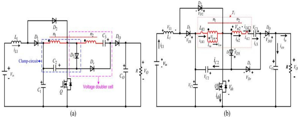
Fig 1: Circuit configuration of proposed converter
