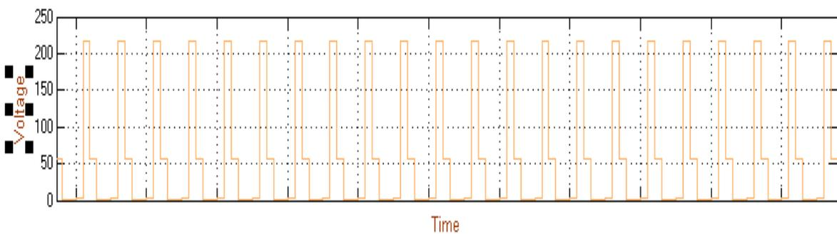
Fig 5(c): Voltage across the switch
