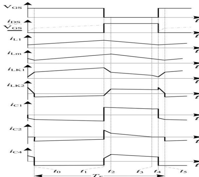
Fig 2 : theoretical waveform in CCM mode
