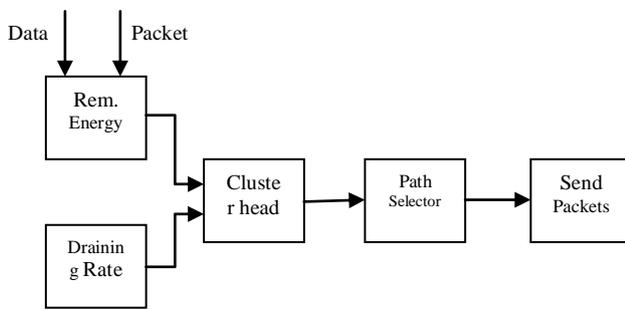
Fig.2 Block diagram for cluster head & path selector
