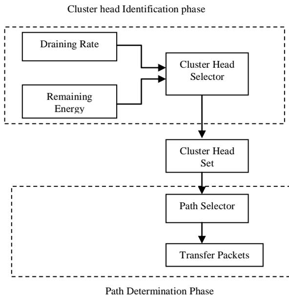
Fig 3: Process model for CH & path selector
