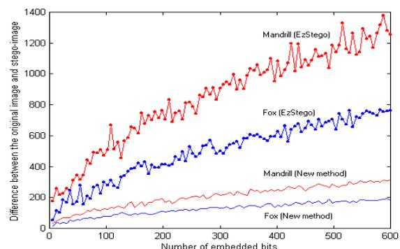
Fig 8 Comparison of distortion introduced by EZ Stego and the new technique.
