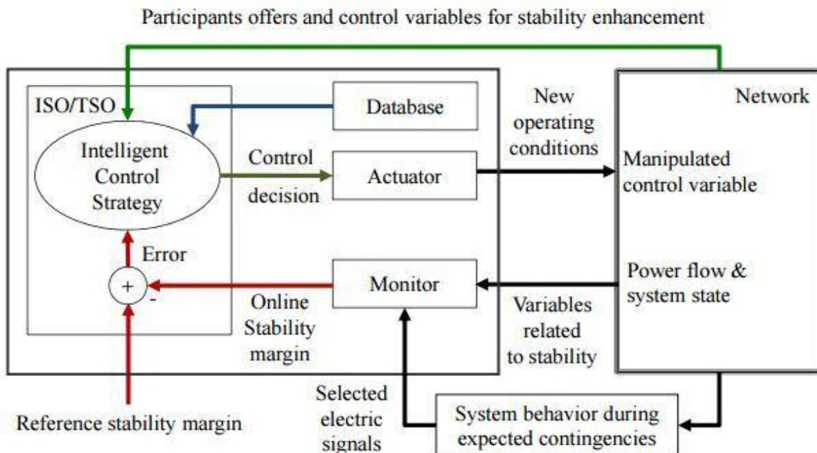
Dynamic system stability is observed based on power system transitory strength and oscillatory stability. Critical fault clearing time (CCT) is used as pointer for TSA and minimum damping of oscillation (MDO) works as indicator for OSA. The values of CCT and MDO at the most believable incident can be used as dynamic stability indices in typical control centers. of Dynamic stability
