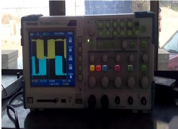
Fig. 7. PWM output of two phase
