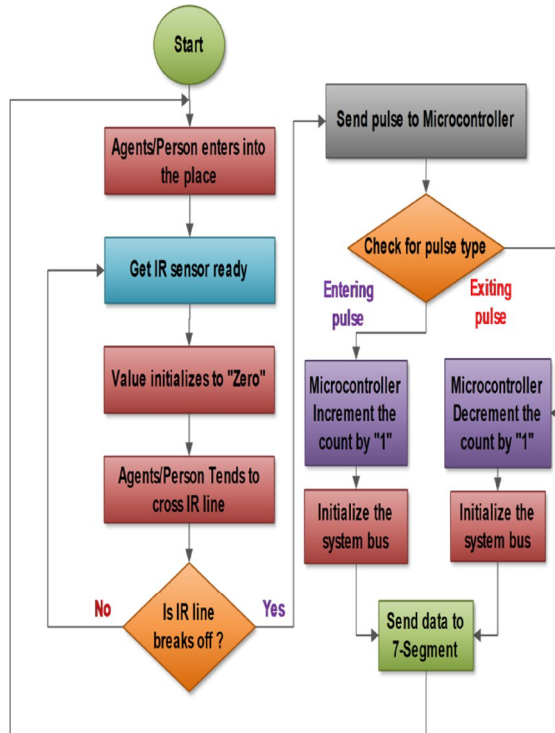
Fig.4 Algorithm for operation
