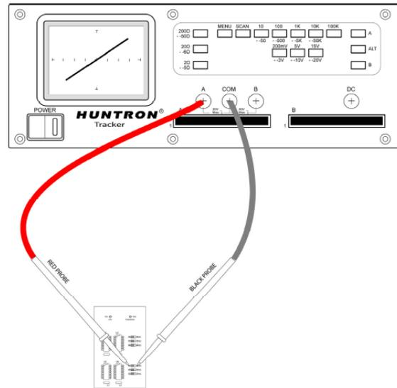
Fig. 6 A typical ASA testing Instrument [3]
