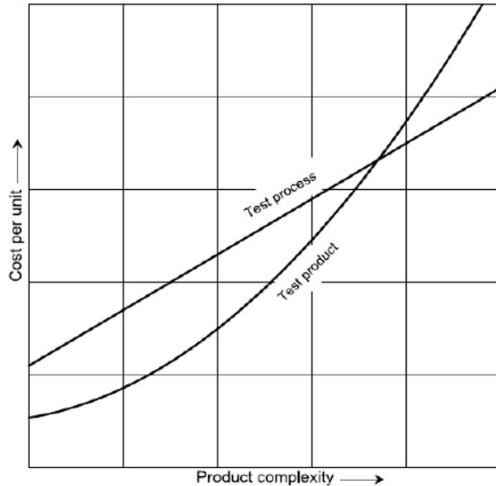
Fig. 1 Test process versus test product [1]
