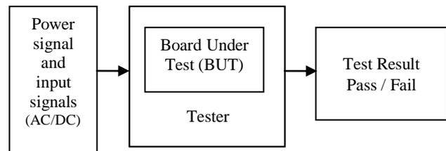
Fig.3 Functional Testing
