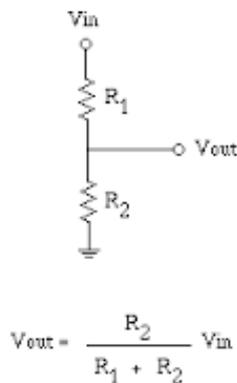
Figure3: Voltage divider
