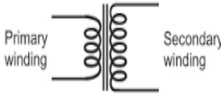
Figure2: Step down Transformer
