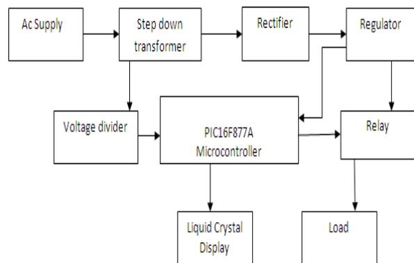
Figure 1: Functional Block Diagram of the Under and Over Voltage Protective Device.
