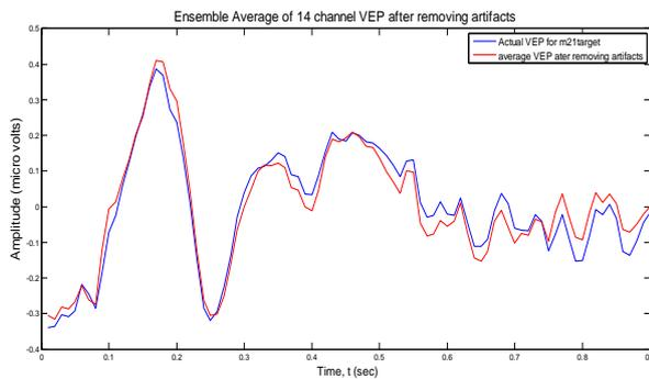
Fig. 4 Comparison of average VEP before and after removal of artifacts for subject m21target
