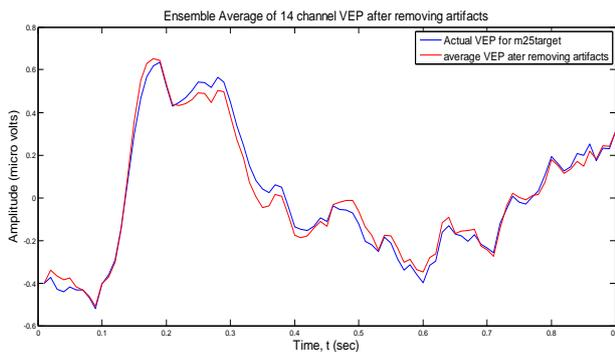
Fig. 5 Comparison of average VEP before and after removal of artifacts for subject m25target
