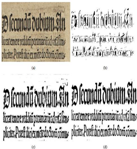
Fig. 3. (a) An old degraded document image; The outputs of (b) Preprocessing, (c) Main Binarization, and (d) Postprocessing.
