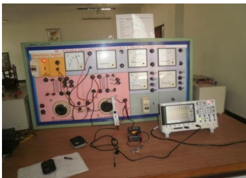
Fig 4 Test Setup to measure inrush current
