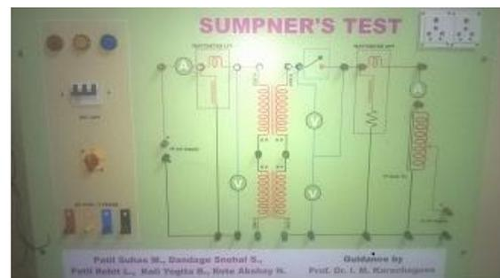
Fig1.2 - Implementation Diagram for Sumpner’s test
