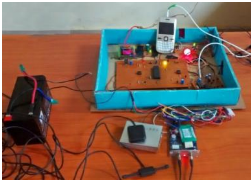
Fig. 5. GPS and GSM system for vehicle.
