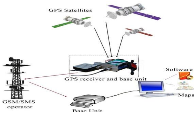
Fig. 6. Block diagram of GPS tracking system.
