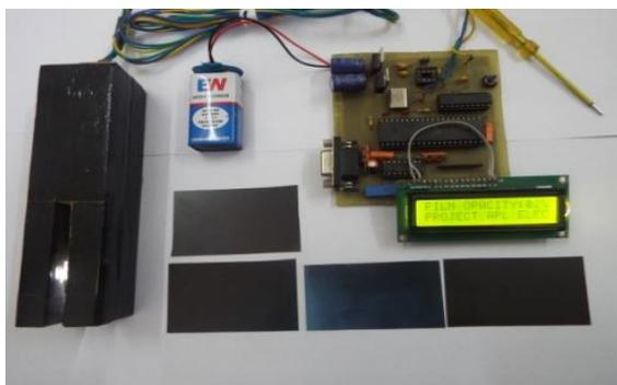
Fig. 4. Complete hardware Setup for experiment
