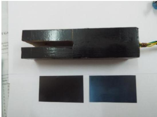
Fig. 3. Opacity Transducer with Film Samples
