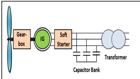
Fig. 2 Schematic diagram of Constant-speed WT
