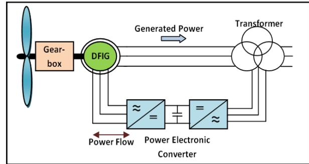
Fig. 3. Schematic diagram of DFIG based WT [36]
