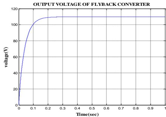
Fig. 12. Output voltage of Flyback converter with R load
