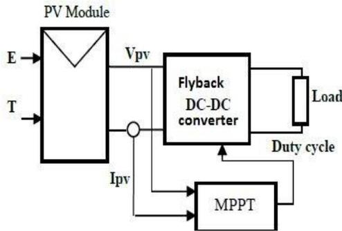
Fig.1.PV with flyback converter and resistive load
