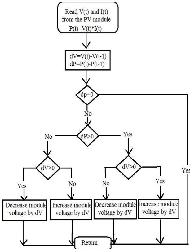
Fig. 6: Flowchart of perturb and observe method
