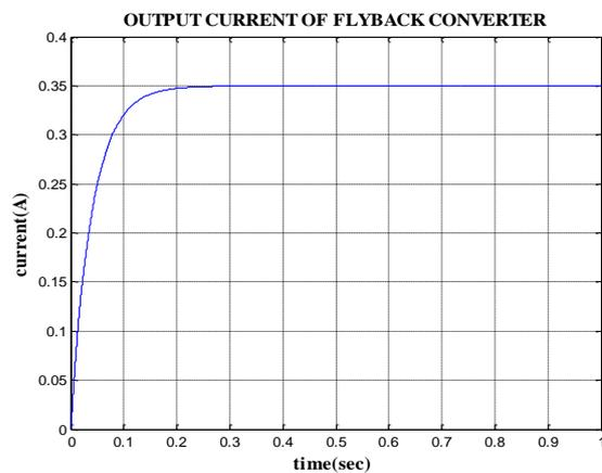
Fig. 13. Output current of Flyback converter with R load
