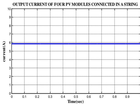
Fig. 9. Output current of four PV modules connected in a string
