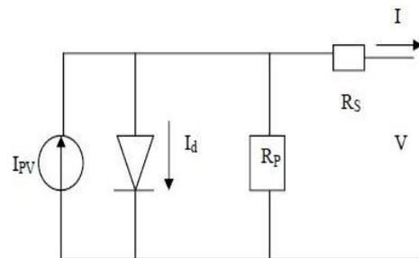
Fig.3: Equivalent model of PV module
