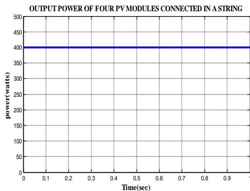
Fig. 10. Output Power of four PV modules connected in a string
