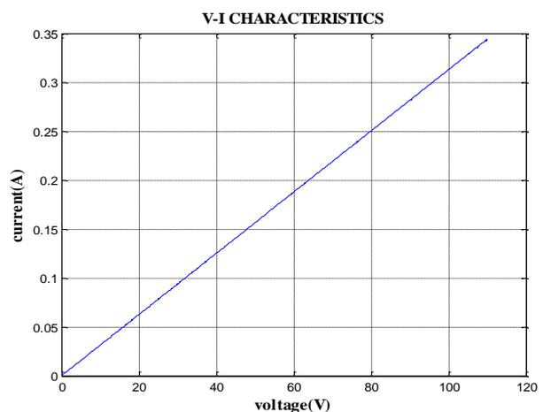
Fig. 14. V-I characteristics of 40W bulb
