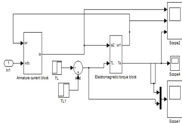
Fig 8: Simulink model of permanent magnet dc shunt motor
