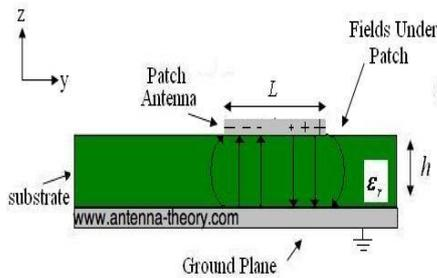
fig 2.(c) side view of antenna resembles field underneath the patch [1]
