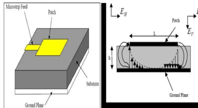
Fig 2.(a) basic elements of patch antenna[1] fig 2.(b) side view of antenna[1]
