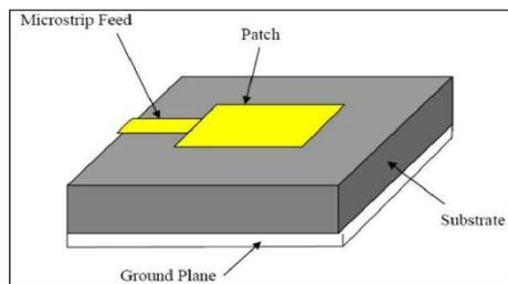
Fig 1 Elements of microstrip patch antenna[1]
