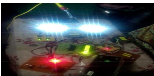
Fig. 7: High-Brightness LED Driver with Film Capacitor
