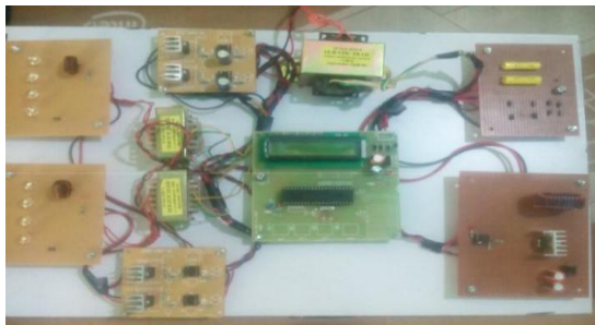
Fig. 6: High-Brightness LED Driver with Film Capacitor
