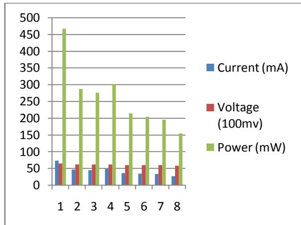
Figure 4.1 Variations of Current, Voltage and Power with Colour Filters
