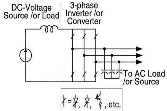
Fig.5. Current-Source Inverter
