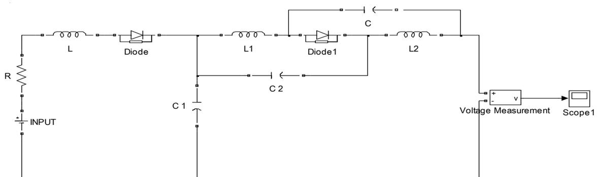
Fig.13.Simulink model of impedance source inverter
