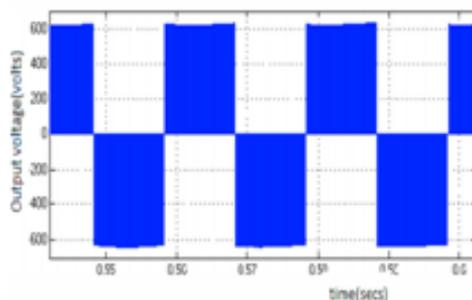
Fig.18.Voltage profile of impedance source inverter
