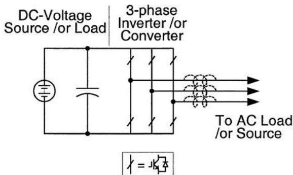
Fig.4. Voltage-Source Inverter
