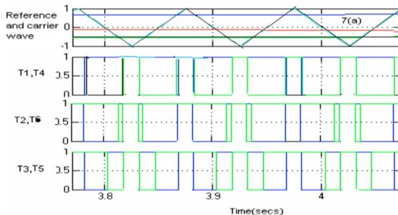
Fig.17.Firing pulses impedance source inverter
