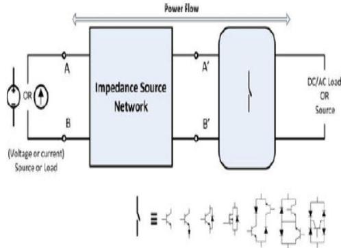
Fig.3. General configuration of impedance source network
