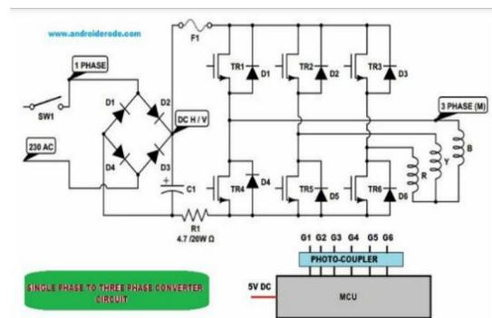
Fig. 7. Single phase to three phase converter
