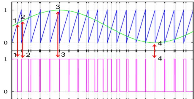
Fig.9. Pulse width modulation
