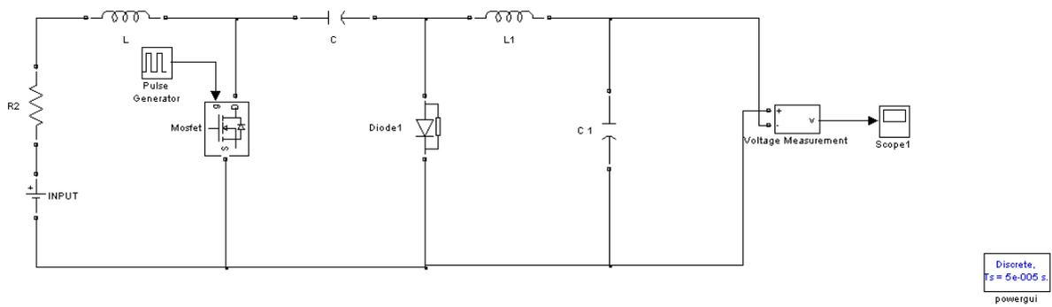
Fig.12.Simulink model of cuk converter
