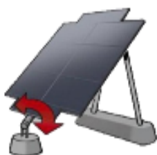
Fig. 2: Single axis tracking system
