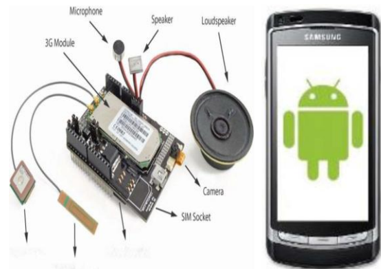
Fig.7. Circuit complexity and size comparison of embedded circuit and android mobile.
