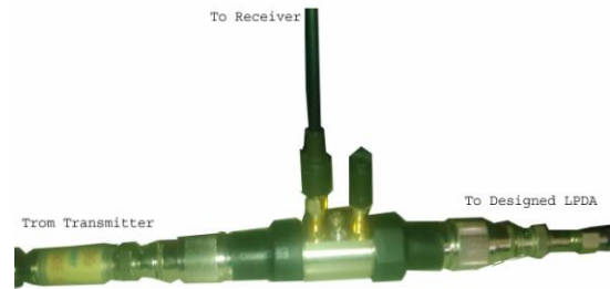
Fig. 8. Connections measurement of incident power
