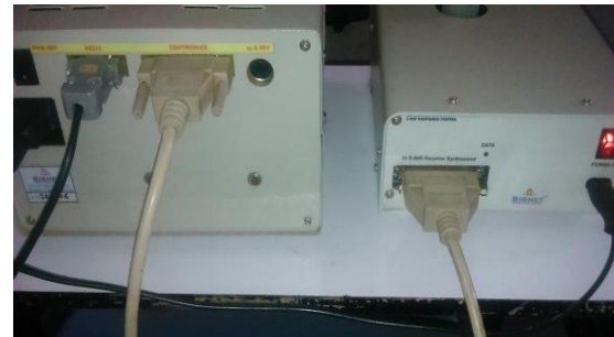
Fig. 4. Stepper motor rotator and S-99R receiver connection
