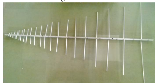
Fig. 1. Photograph of constructed LPDA
