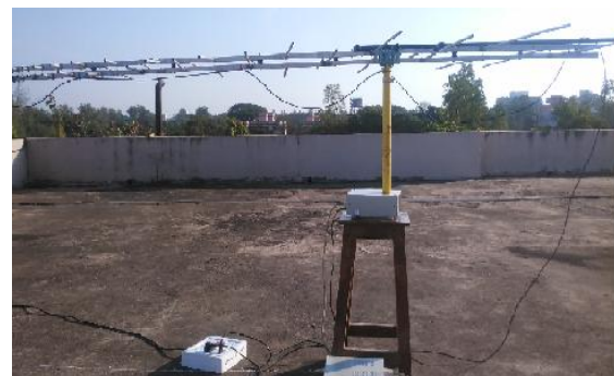
Fig.5. Arrangement of LPDA and stepper motor
