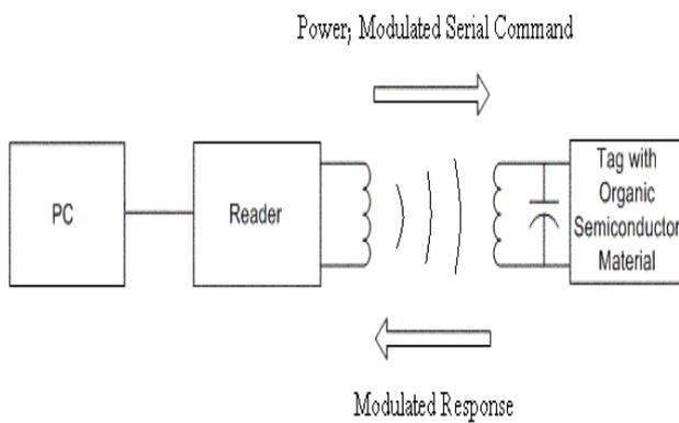
Block diagram of RFID
