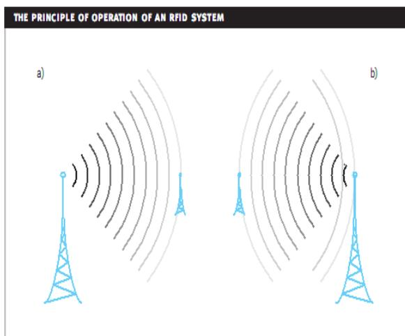
Principle of operation of an RFID
