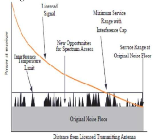
Fig 6. Model for Interference Temperature
