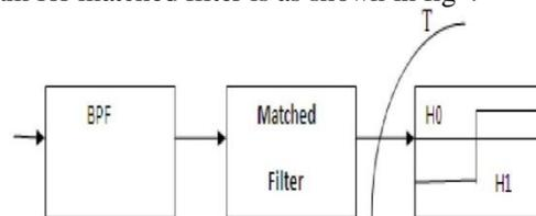
Fig 4. Block Diagram for Matched Filter Detection
