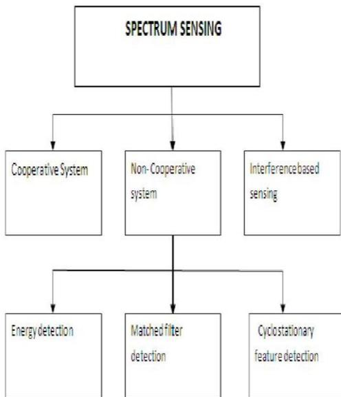
Fig 2. Spectrum Sensing Techniques
