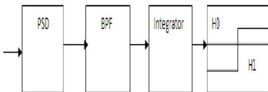
Fig 3. Block Diagram for Energy Detection
