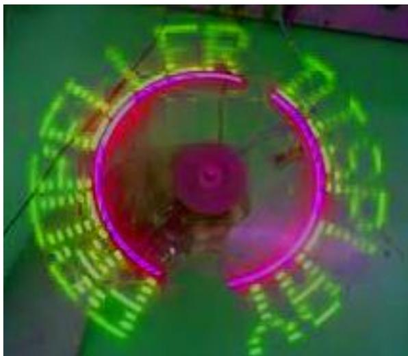
Figure 8: Output of Propeller LED Display
