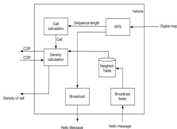
Figure 1:Overview of cell density based traffic information system.
