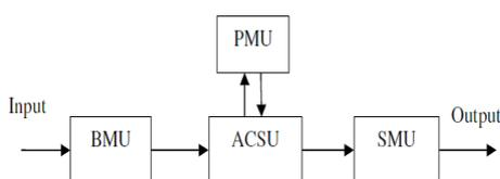
Fig 3. Block diagram of Viterbi decoder
