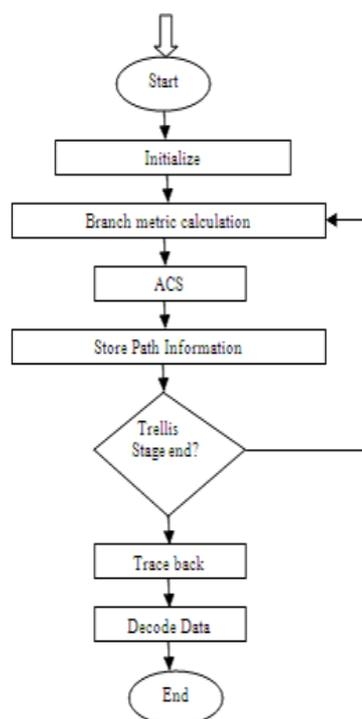
Fig 4: Viterbi decoding Flow Chart
