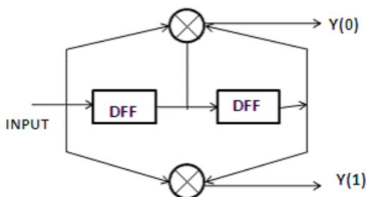
Fig 2. Convolutional encoder
