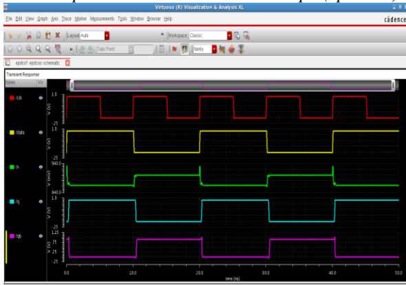
Fig .7 Output waveform of ep-DCO
