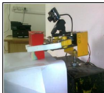
Fig. 1. A simple pick and place robot
