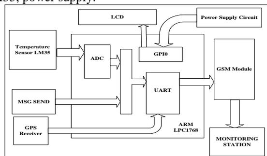
Fig. 1. Block diagram of the Vehicular Monitoring and Tracking System
