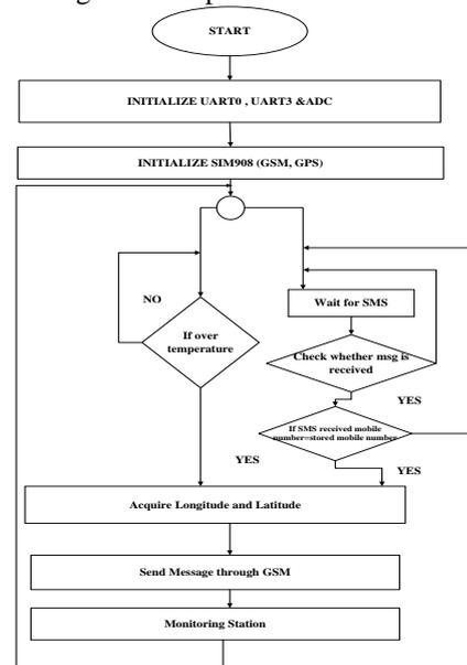
Fig. 6. Flowchart of Vehicular Monitoring and Tracking System
