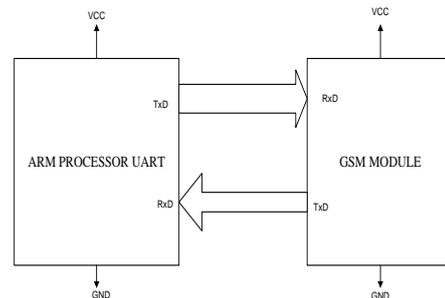
Fig. 5. GSM interfaced with UART of ARM processor
