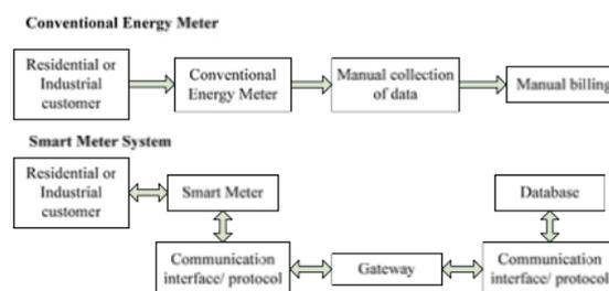
Fig. 1. Architectural model of conventional energy meter and smart meter [1]
