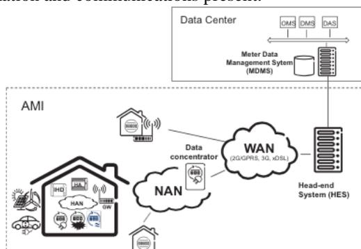
Fig. 3. Basic architecture of an AMI [5]
